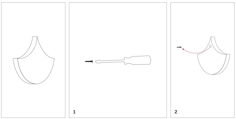
Place one screw into the wall surface.
