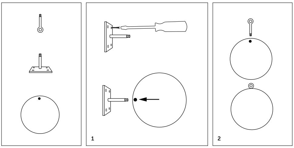
Attach the wall hanger on wall surface using screws.
